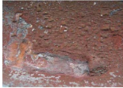
Figure 5. The configurations of the metallic floor pipe sample after mechanical elimination the eroded offspring
